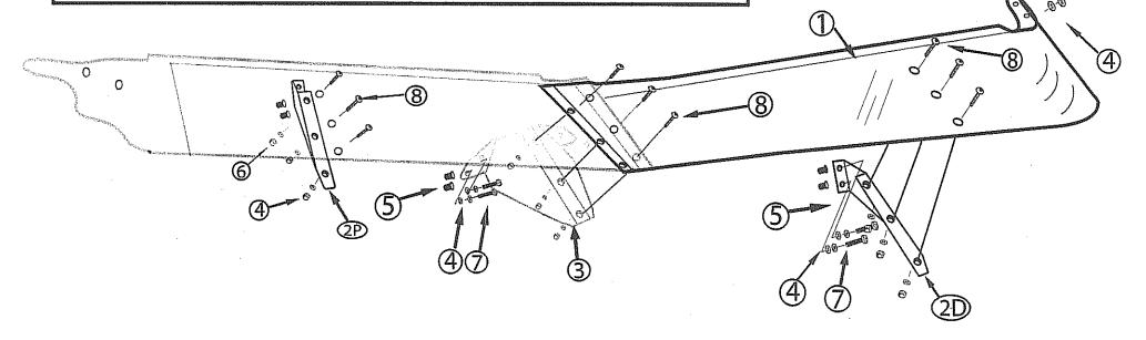
\* Use Lock Washers on all bolts that mount directly to truck cab to prevent loosening due to road vibrations
