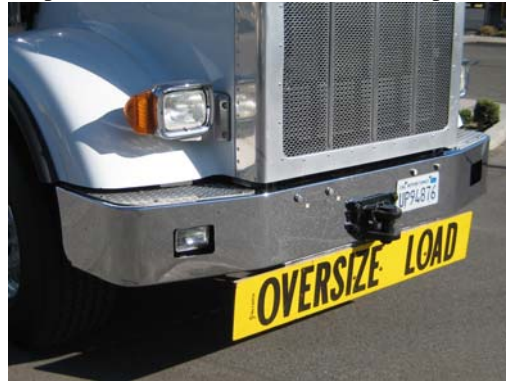
Step 4: Re-install all brackets onto bumper
