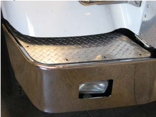
Step 3: Remove diamond plate for re-use
