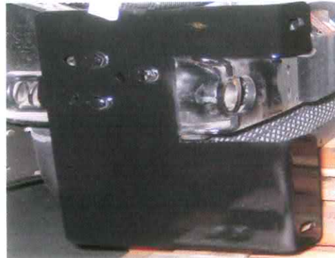
Step 3: Install Brackets (psgr side shown)
